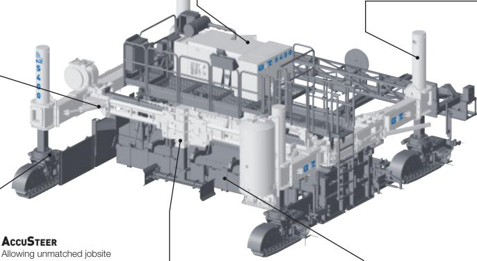
maneuverability, the AccuSteer system utilizes slew drive technology to steer the machine.
