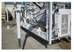
With the use of the DBI Loading stands, the DBI can be loaded without the use of a crane.
