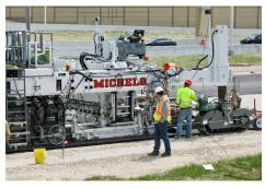
The bolster extensions allow the S400 to continue to utilize its swing legs and maintain a narrow overall width for tight track line situations.
